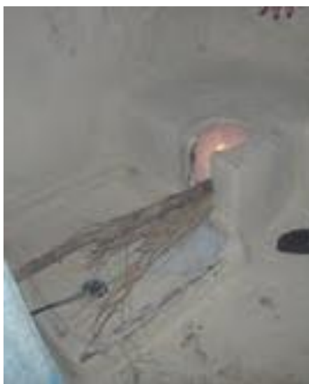
Illustration 4: Mud and brick cookstove used in Polay Kalan, Kalapipal, Shajapur, Madhya Pradesh
